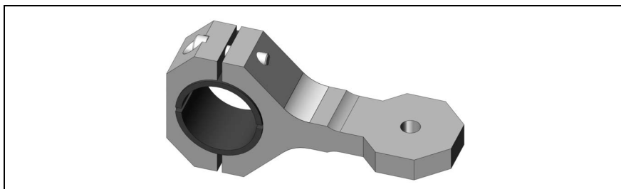
Fig. 3 Mount for the machine cutting torch
