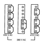
manual or the digram attached to the inside of the access door on the left side of the machine for correct positioning of the jumper links of the primary terminal board. Unused jumper links should be placed in parallel with a used jumper to prevent loss of the unused link.
